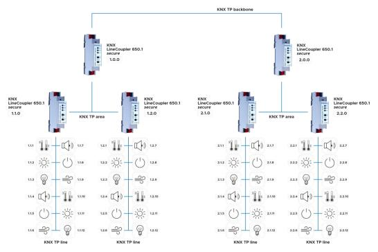
The individual address of the KNX LineCoupler 650.1 *secure* corresponds to the form x.0.0 (x: 1 ... 15). Thus the device functions as area coupler.
