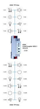
The individual address of the KNX LineCoupler 650.1 *secure* corresponds to the form x.y.z (x, y: 1 ... 15, z: 1 ... 255). Thus the device functions as repeater.
