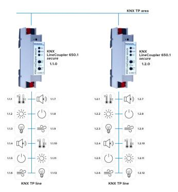
The individual address of the KNX LineCoupler 650.1 *secure* corresponds to the form x.y.0 (x, y: 1 ... 15). Thus the device functions as line coupler.
