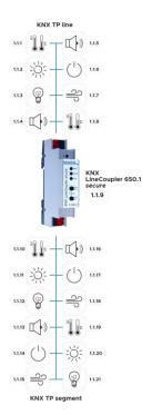
The individual address of the KNX LineCoupler 650.1 *secure* corresponds to the form x.y.z (x, y: 1 ... 15, z: 1 ... 255). Thus the device functions as segment coupler.
