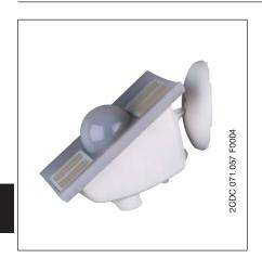
The weather sensor WES/A 1.1 is used primarily for domestic purposes. For detection of twilight (1...999 Lux), brightness in three directions (1,000...99,000 Lux), rain (upper sensor and lower surfaces are permanently heated. Temperature (– 30...+50 °C), day/night, windspeeds (0...24.0 m/s), date and time (DCF radio receiver). An additional heating transformer is not required. The Weather Sensor WES/A 1.1 works only in conjunction with the WZ/S 1.1 Weather Unit.
