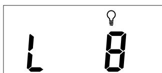
③ Switch to the desired level of brightness from 0 (dark) to 9 (bright) by pressing the left or right key on the display (Figure ⑪)
